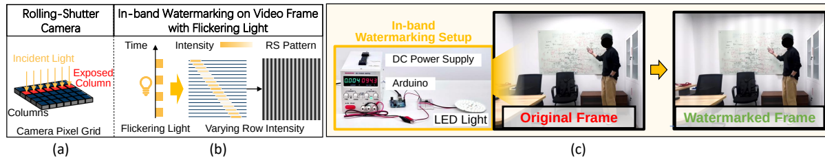
Fig. 5. Figure depicts that (a) a rolling-shutter camera exposes the image line by line. (b) When illuminated by a modulated light source, each column of pixels integrates a slightly different light intensity over time, resulting in vertical stripe patterns that encode the watermark signal within the captured frame. (c) Implementation setup of LightMark's in-band watermarking system , consisting of a DC power supply, an Arduino controller, and an LED light source. The modulated light embeds authentication data into the captured scene, producing watermarked frames for subsequent validation.
