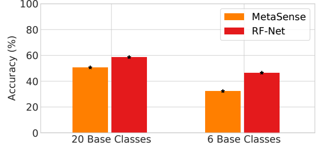
Figure 2: Accuracy of MetaSense and RF-Net to recognize unseen gestures. Neither of them can achieve acceptable accuracy with a small base dataset.
